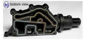
Fig. 4. K4M engine thermostat assembly
